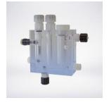
Bleed-off control - Controls the accumulation or buildup of dissolved solids in the recirculating water caused by the evaporation. The bleed-off control operates a bleed-off valve to drain water from the system, allowing additional make-up to dilute the system water and reduce the dissolved solids level.
